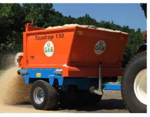
The Topdrop is a premium brush dresser, with which you can accurately apply several materials. By means of a conveyer belt, the sand is transported to the mechanical adjustable metering valve. Since the brush is hydraulically powered, the quantity of material applied can accurately be determined.
