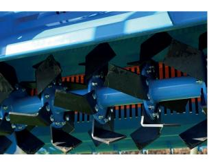
The Stoneburier is a premium rotary tiller, in which the strainer behind the rotary tiller ensures that the stones get separated from the finely crumbled ground. It is possible to equip the rotary tiller with two different types of tilling blades. Because of this operation the stones will be put under the layer of fine, vital soil.
