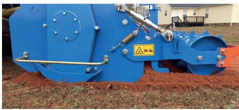
The maximum operating depth of the Stoneburier is 17 cm. The operating depth can simply be adjusted by using two spindles on both sides of the machine. The rear roller presses the milled material, additionally, you can fill this roller with water when you want to press the soil more firmly. Optionally the roller can be hydraulically adjusted, so you can seamlessly continue with your operation without stopping.
