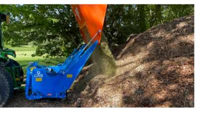
The VCollector is optimally equipped for removing weeds thanks to the CombiRotor. This is a powered rotor developed for scarifying and milling. The rotor rotates against the direction of travel, so that it makes a powerful cutting movement and does not skip a centimeter. With the VCollector, the blades are mounted with wind vanes. This creates an airflow that sucks the milled material into the collection container.
