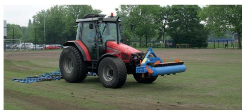
After the tillage, for instance with the Ecodresser, the pitch will be levelled perfectly by the Dragframe. Optionally we can provide the Dragframe with welded mesh panels, so that you can also use the Dragframe on sand. Subsequently, you are in position to work effective and efficient on several surfaces.
