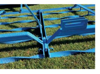
The Dragframe is provided with two folding side decks, which broaden the operating width to 4 m and that can be folded away by an optional hydraulic system. The spiral shaped bars of the Dragframe are developed in such a way that they ensure an even result of your operation.
