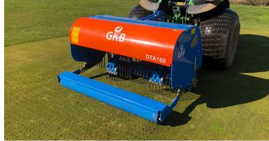
Featuring a 3-speed heavy duty gearbox, you can adjust the speed of the tines to create the required hole pattern in the turf.
